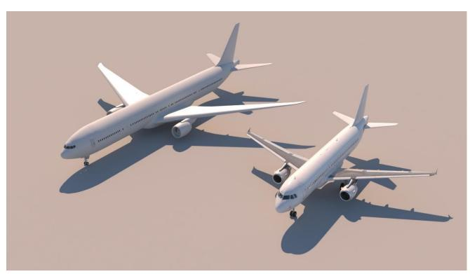
Figure 6.5 Scale of the B777 (left) and A320 (right) planes
