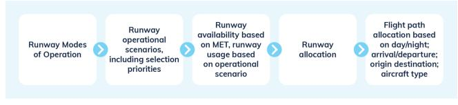
Figure 11.6 Process to allocate a WSI flight operation to a runway and flight path
