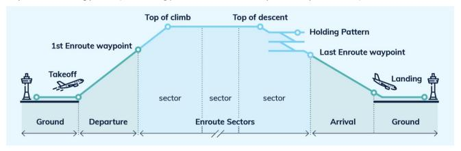
Figure 3.11 Phases of flight
