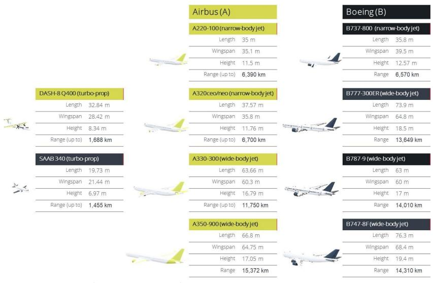
Figure 2.4 Size comparison of selected representative aircraft at WSI
