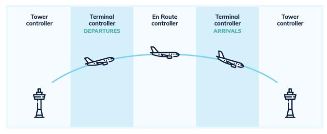
Figure 3.2 How air traffic control works
