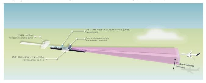
Figure 3.9 Instrument landing system
