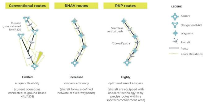
Figure 3.10 Conventional airspace routing versus RNAV and RNP routing
