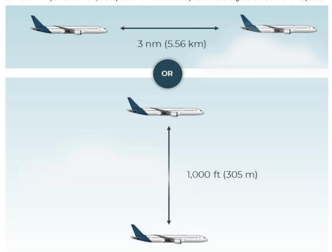
Figure 3.16 Separation distances for IFR aircraft
