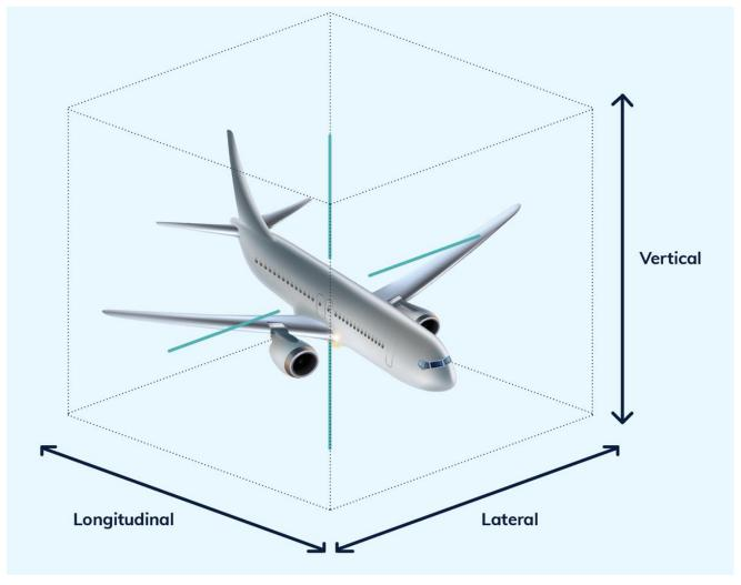
Figure 3.1 Three-dimensional space in which aircraft fly
