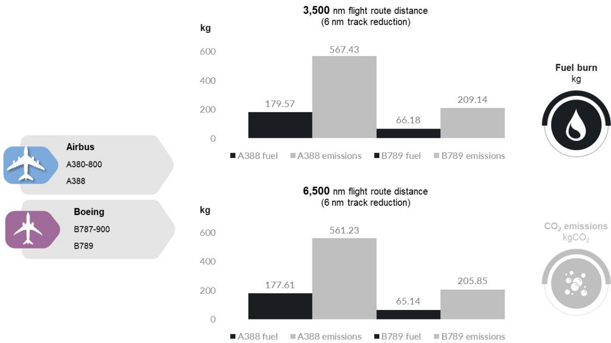
Figure 8.1 Fuel consumption and CO 2 emissions per movement for selected widebody jet aircraft types
