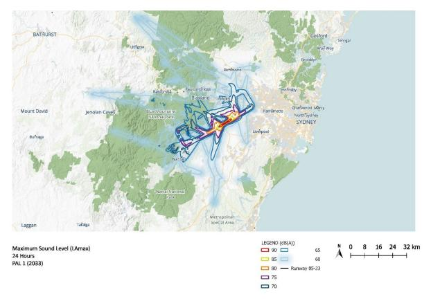
Figure 9.38 L<sub>Amax</sub> 24-hour contours (cumulative) – 2033
