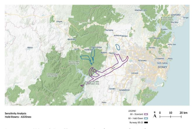
Figure 9.35 Sensitivity analysis – Hold Down – comparison of L<sub>Amax</sub> contours (A320neo)
