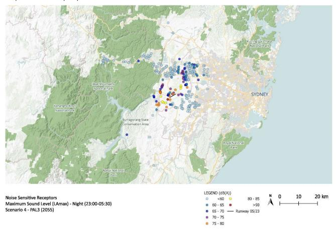
Figure 9.19 Noise sensitive receptors (NSR) – maximum sound level (L<sub>Amax</sub>) – Night – scenario 4 – 2055 (PAL 3)
