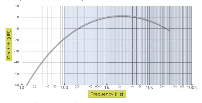
Figure 3.1 Sound pressure level – A-weighting
