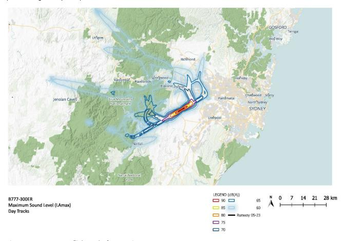
Figure 9.41 L<sub>Amax</sub> Day flight paths for a Boeing B777-300ER
