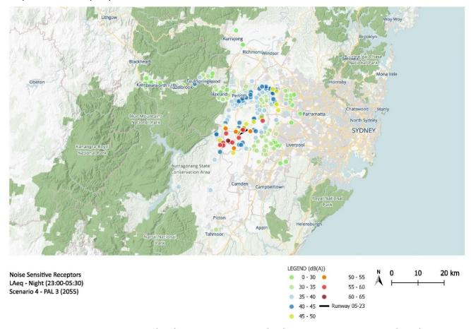
Figure 9.17 Noise sensitive receptor (NSR) – Average sound level (LAeq) – Night – scenario 4 – 2055 (PAL 3)
