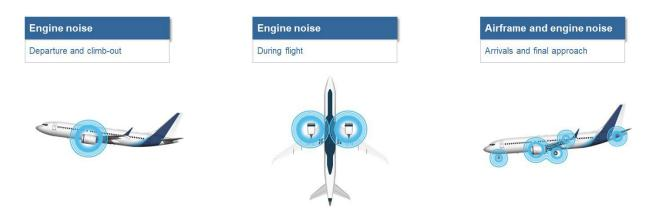
Figure 3.3 Noise sources from an aircraft in flight
