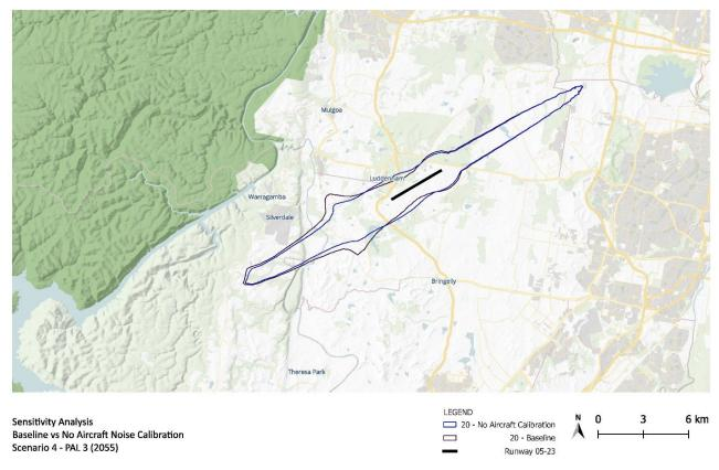
Figure 9.34 Sensitivity analysis – aircraft noise calibration – comparison of 20 ANEC contours
