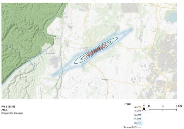
Figure 9.7 Example ANEC contour – composite scenario in 2033 (PAL 1)
