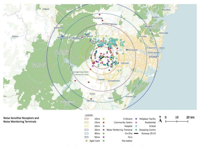
Figure 9.15 Noise sensitive receptors (NSRs) and noise monitoring terminals (NMTs)
