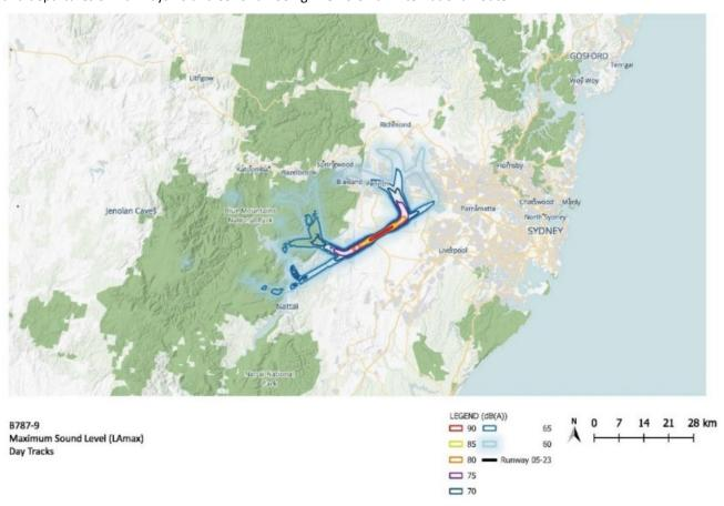
Figure 9.9 Example single event noise contour for Boeing B787-9 Day flight paths (5:30 am to 11 pm)
