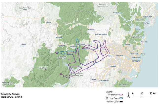
Figure 9.36 Sensitivity analysis – Hold Down – comparison of L<sub>Amax</sub> contours (B787-9)
