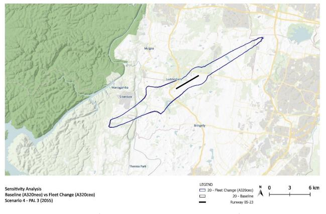
Figure 9.30 Sensitivity analysis – fleet mix A320ceo versus A320neo – comparison of 20 ANEC contours
