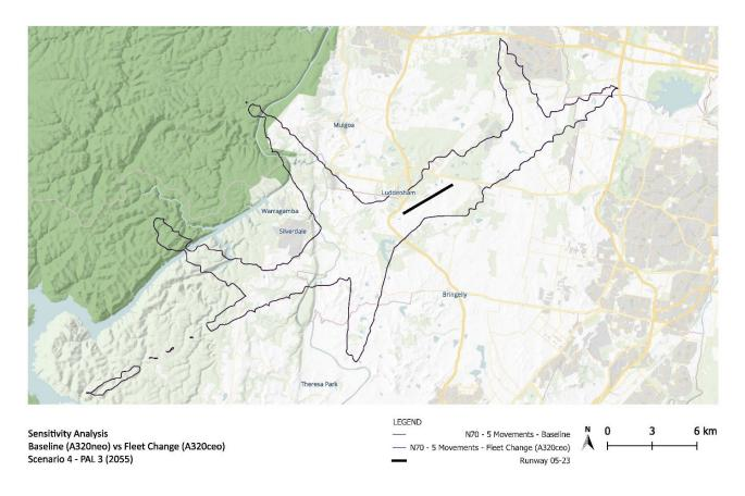
Figure 9.29 Sensitivity analysis – fleet mix A320ceo versus A320neo – comparison of N70 contours – 5 movements
