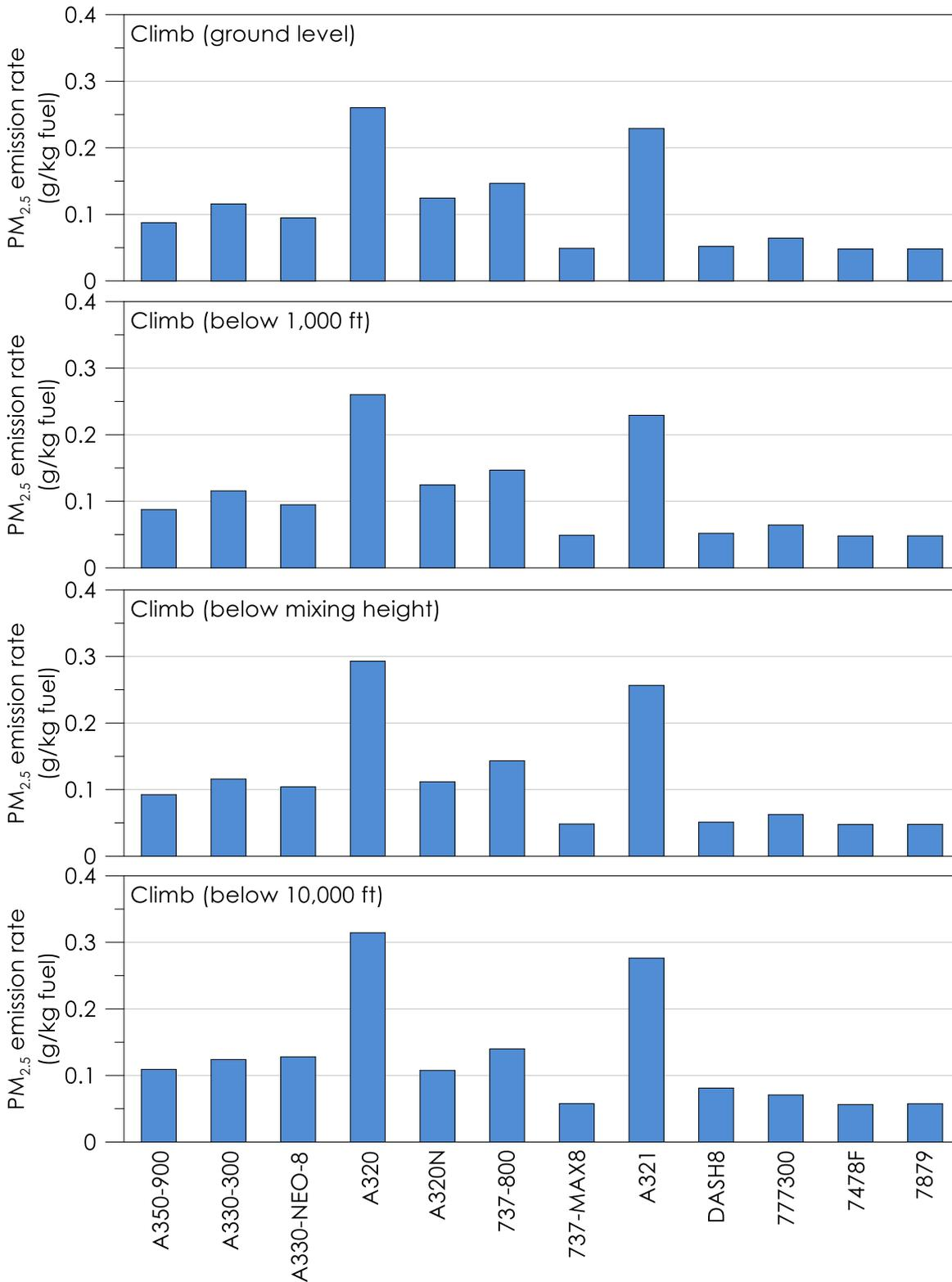
Figure 5.7 Estimated PM<sub>2.5</sub> emissions rate for aircraft during departure
