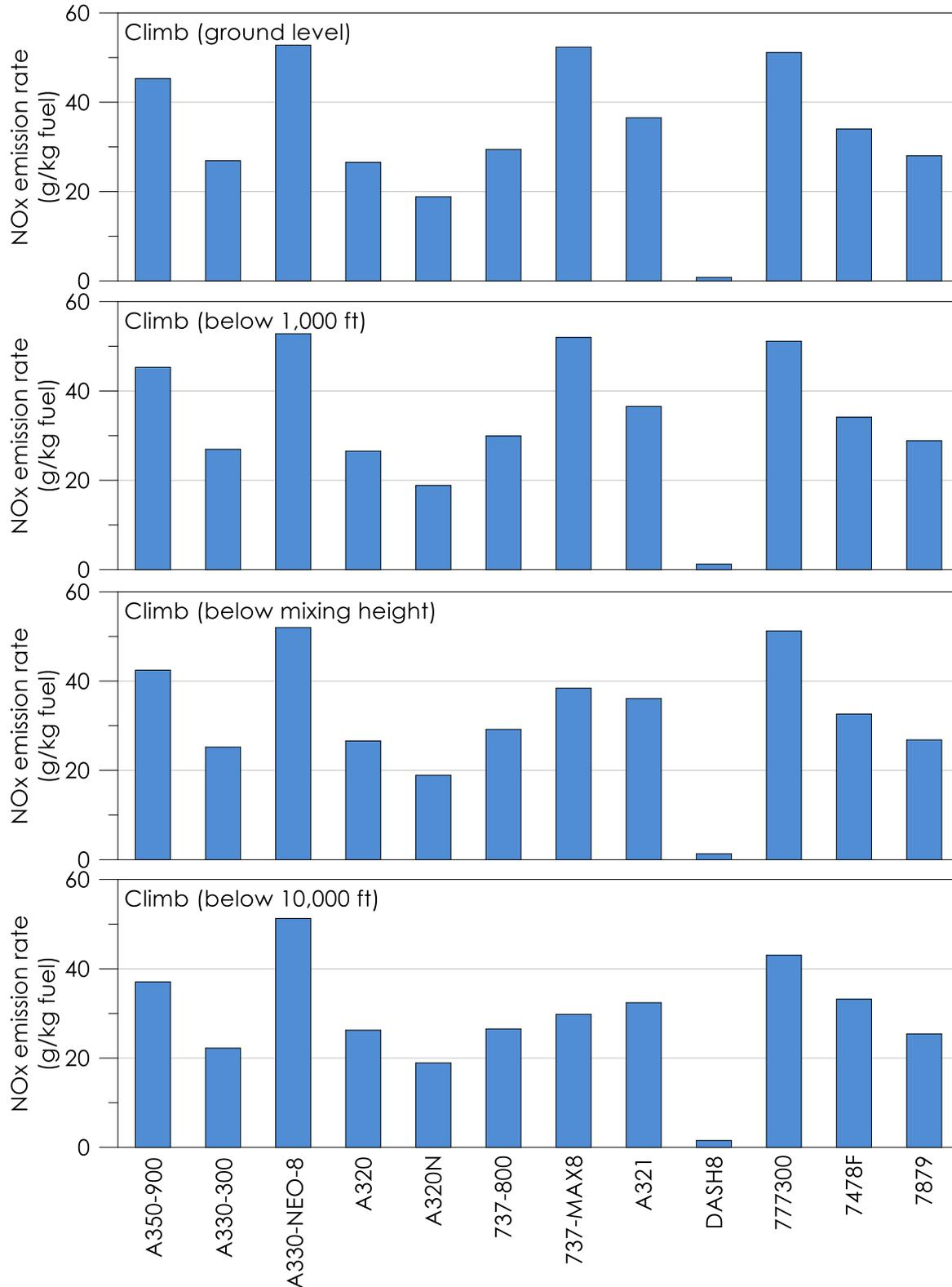
Figure 5.5 Estimated NO<sub>x</sub> emissions rate for aircraft during departure
