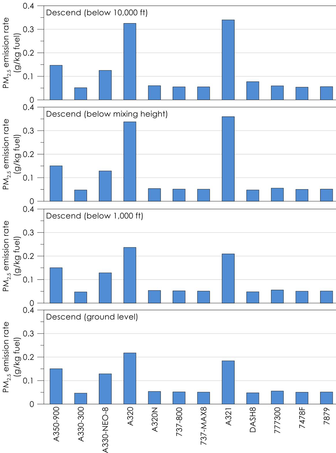
**Figure 5.8** Estimated PM<sub>2.5</sub> emissions rate for aircraft during arrival
