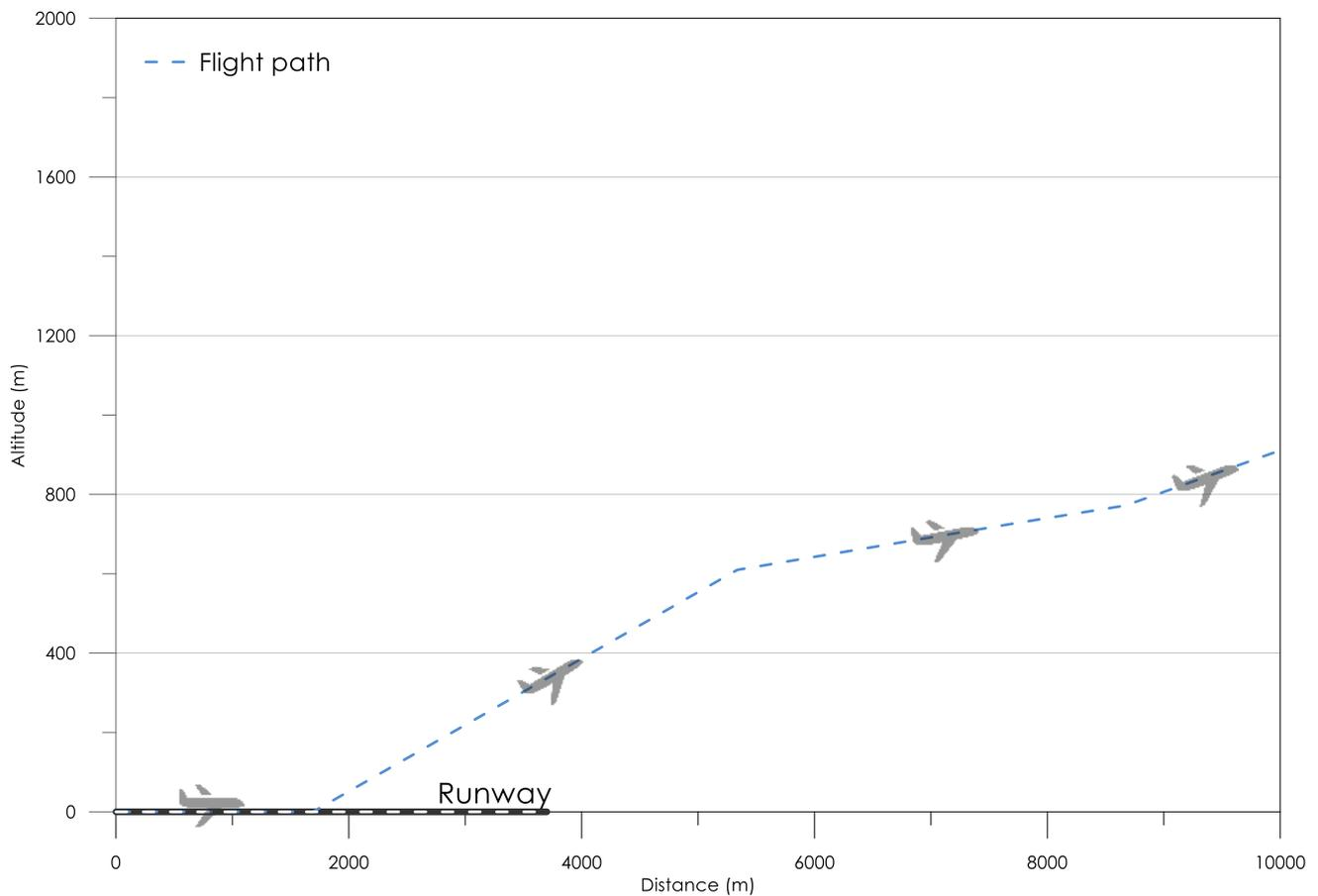
**Figure 5.3 Typical vertical profile of a departing flight path considered for the assessment**
