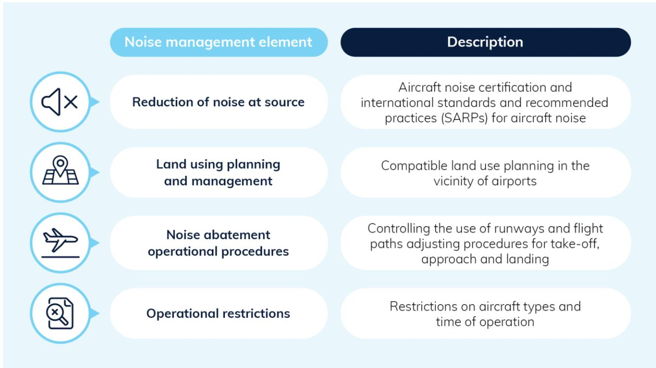
**Figure 11.3 ICAO’s Balanced Approach to Aircraft Noise Management**
